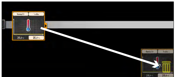
Fig. 5 To delete a parameter icon from an editor thread, drag the icon, with the mouse button depressed, to the recycle bin symbol.
