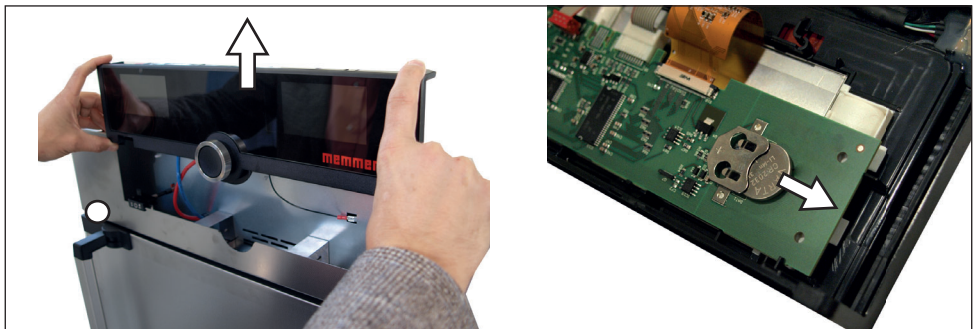
Fig. 23 Removing the lithium battery
