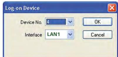
If an interface was specified and CELSIUS cannot find an oven at this interface, this setting is switched automatically to offline. CELSIUS automatically determines the configuration of ovens connected online.
