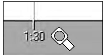
► Move the mouse cursor over the vertical axis in the temperature, humidity, pressure, CO<sub>2</sub> or O<sub>2</sub> windows. The mouse cursor turns into a magnifying glass. You can now
