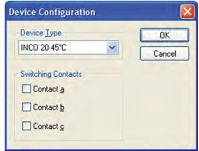
Select from the list the oven type that you want to simulate or to which you want to transfer a tempering profile, and confirm this with "OK". With optional extras (e.g. additional switching contacts), these must be activated manually for them to be used later on.
