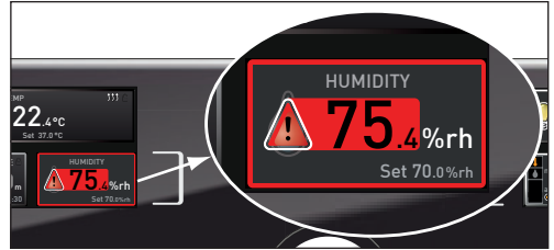
Fig. 22 Humidity monitoring triggered
