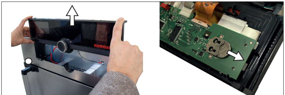
Fig. 41 Removing the lithium battery
