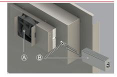
ance B. The cooling function switches on immediately (fan is running) and regulates itself. You can attach the power supply unit to the appliance using the Velcro fastener provided.
