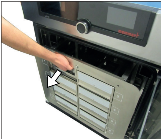
Fig. 8 Pull the slide in unit out of the drawer opening
