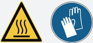
During operation of the pumping device, individual components may heat up. Touching its surface can cause burns. Use temperature-resistant protective gloves.
